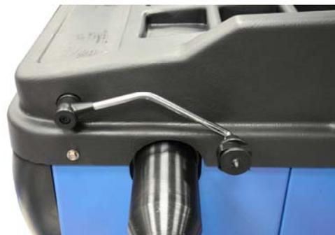
**STEP 12:** The display will read “d-t 200”. Using a metric ruler, measure “200mm” (20cm) directly up (**vertically**) from the top of the balancer’s main shaft as shown.
