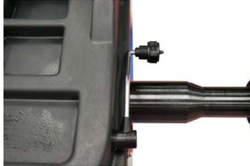
**STEP 9:** The display will read “A-t 200”. Move the gauge to the “200mm” (20cm) position as shown. While the gauge is held at the “200mm” position, press “ENTER” to save the setting in the balancer’s memory.
