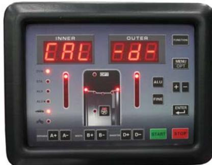
**STEP 11:** The display will read “d-0 0”. Set the gauge at the “0mm” (fully closed) position as shown. While the gauge is held at the “0mm” position, Press “ENTER” to save the setting in the balancer’s memory.
