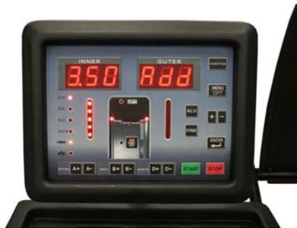
**STEP 10:** When the cycle is finished, the display will read “Add 3.50” (100 grams). Remove the calibration weight from the inside edge of the wheel. Rotate the wheel until all the outside weight indicators are fully lighted. Apply the 3.5 ounce (100 gram) calibration weight to the outside edge of the wheel at the 12 o’ clock position. Lower the hood and spin the wheel.
