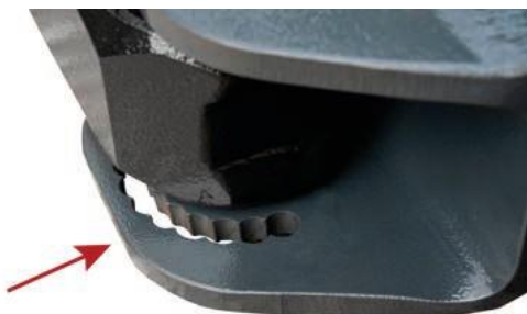
Fig. 25: Layout of holes for adjusting the support arms
