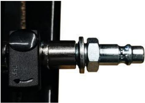
Fig. 16: Compressed air connection installed
