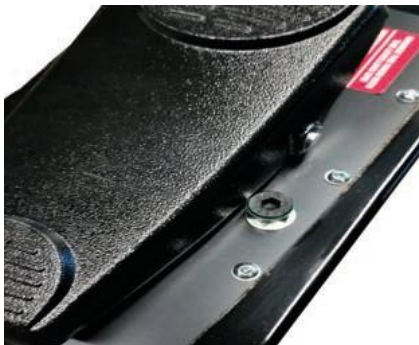
Fig. 21: Oil filler connector with dipstick
