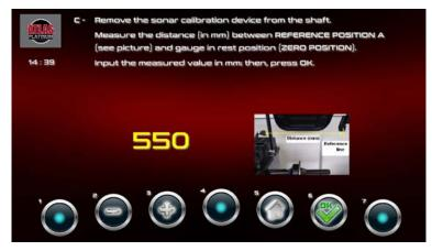
Measure the distance (in mm) between the reference line on the sonar and the distance gauge <u>clip</u> in rest position (ZERO POSITION)
