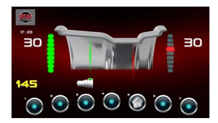
Pull out the gauge until the counterweight applicator reaches the previously selected area, FI or FE.
