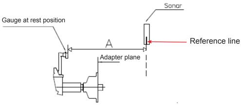
Insert the distance measured in mm using the display, 550 (mm).
